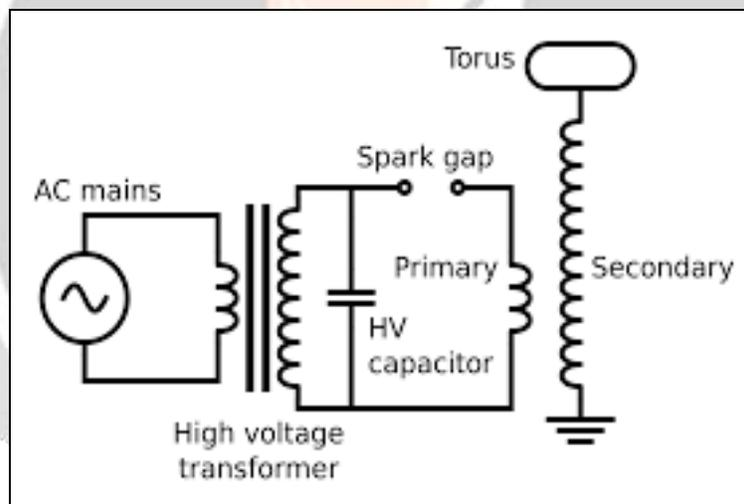
Fig 1. Typical Tesla coil circuit [6]
