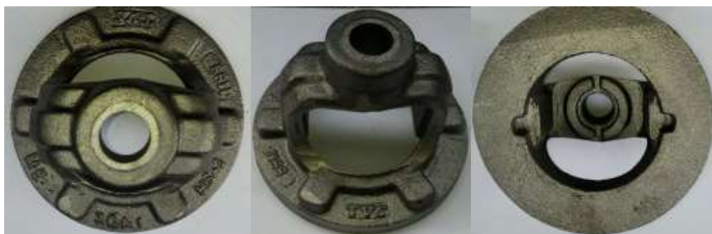
Fig. 15 Final Accepted Defect Free Casting of TVSSATELITE
