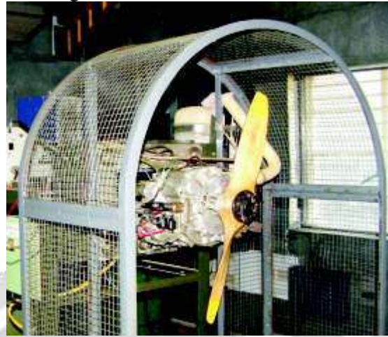
Fig.3 Rotary Engine on test set up
