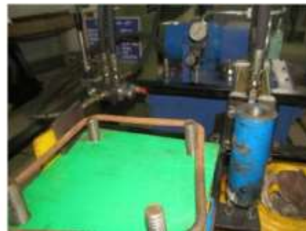
Figure 1.9 Stirrup bent by the machine
