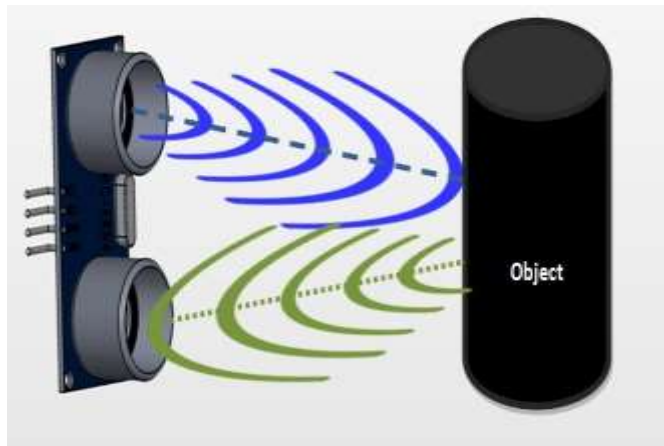
Fig.3 HC-SR04 ULTRASONIC SENSOR - WORKING
