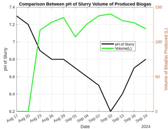
**Chart -2:** How pH of slurry affects the volume of biogas produced
