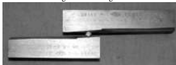
Fig.1. Flat rolling die.
