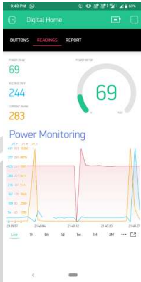
Fig.4 Power Monitoring in Blynk App
