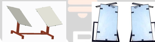
Fig -4: Designed & Fabricated Tracking System with Mirrors
