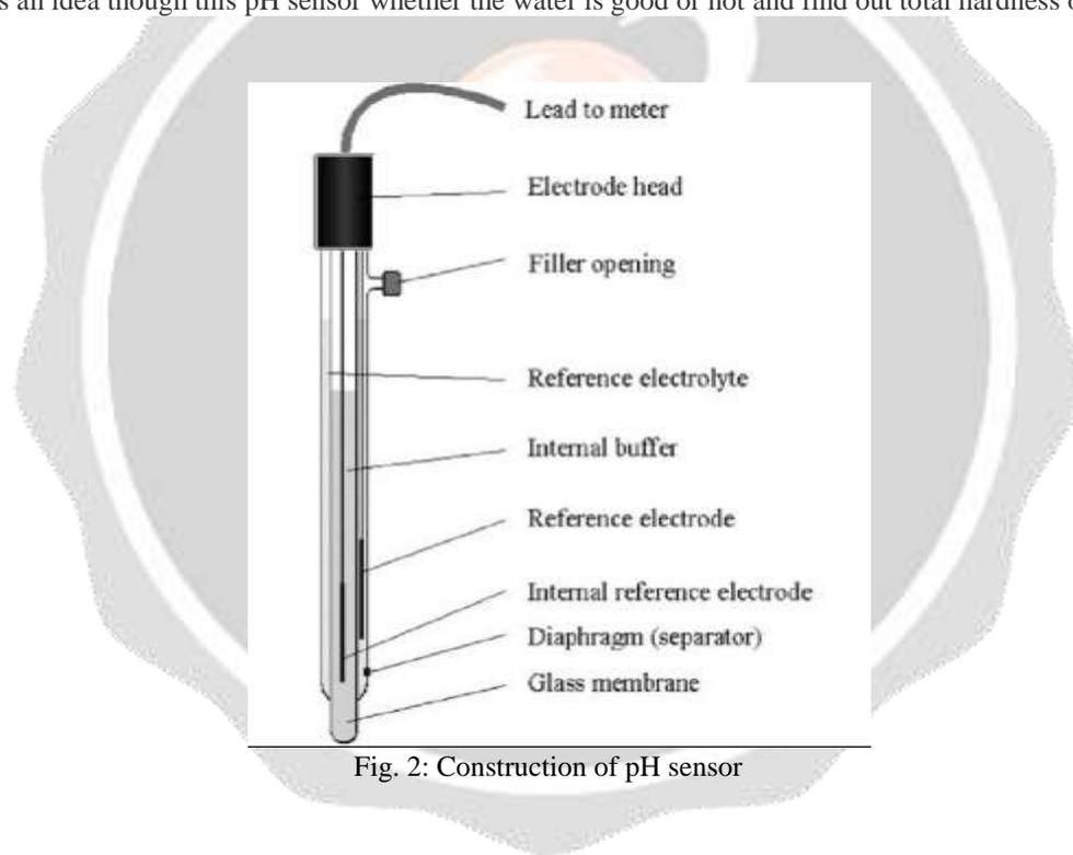
Fig. 2: Construction of pH sensor
