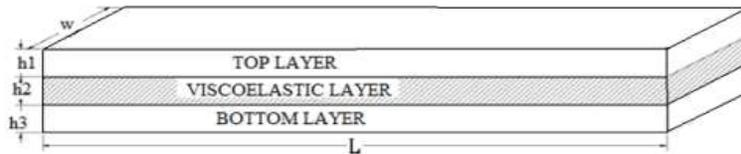
Figure: 3.2 Viscoelastic sandwich beam
