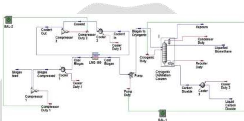
**Fig. 2.** Design of a liquefaction process of biogas in Aspen HYSYS
