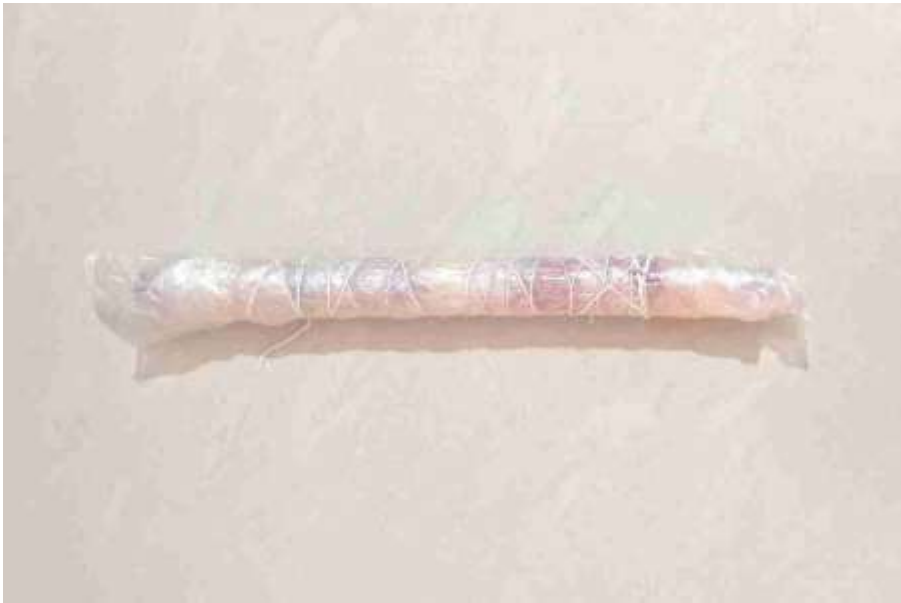
Fig:4.5 (Ties with plastic sheet)
