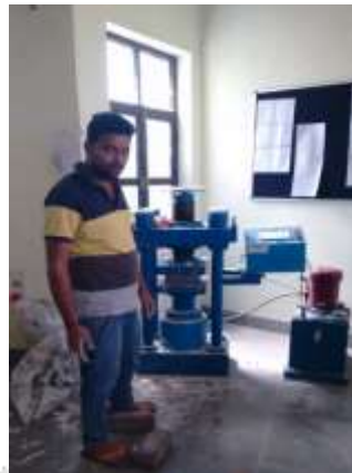
Figure 2: Setup of Compression Strength Test
