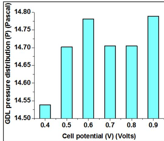
Fig -3: GDL pressure distributions for all cell voltages
