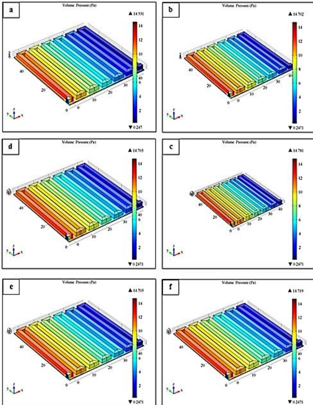
Fig-2: GDL pressure distribution at cell potential (a) 0.4V (b) 0.5V (c) 0.6V (d) 0.7V (e) 0.8V (f) 0.9V
