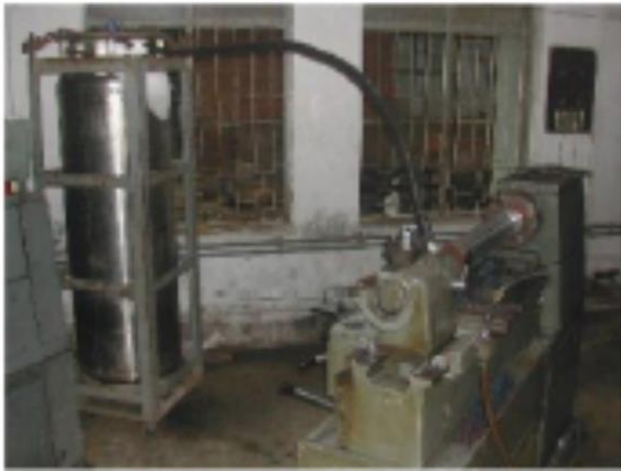
Fig. 8. Photograph view of the experimental set-up for turning Nozzle injection liquid nitrogen steel with liquid nitrogen.
