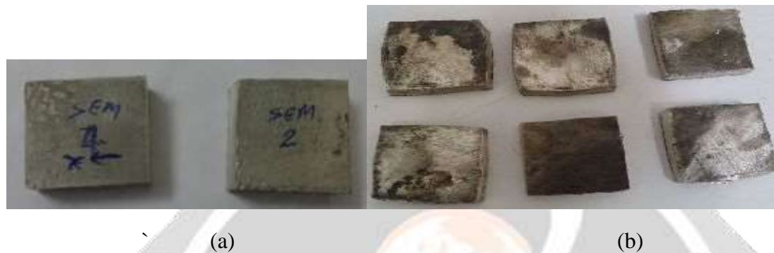
Figure 2.1: Sample(a) before forging, (b) After forging
