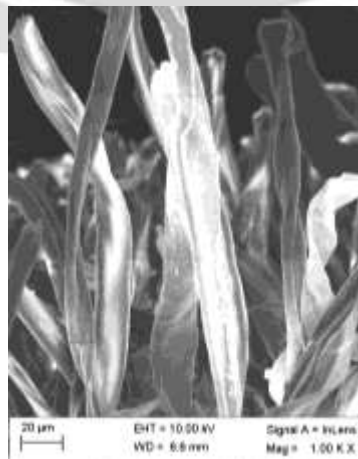
Fig:6.2.5 (SEM analysis of plasma treated fabric of electrode distance 8cm for 15mins)
