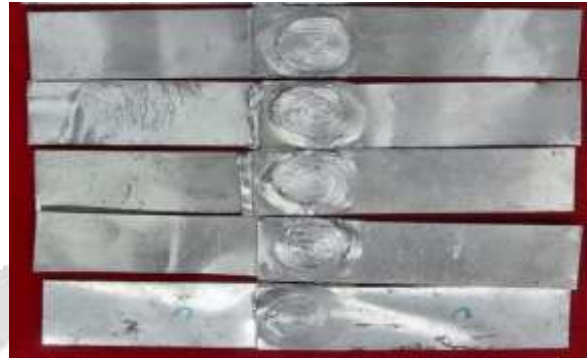
Fig-4: FSMB by altering tool rotation speed.
