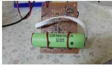
Fig. 8: MH12210 Lithium Ion battery
