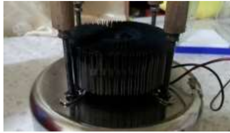
Fig. 5: Aluminum heat sink as hot side
