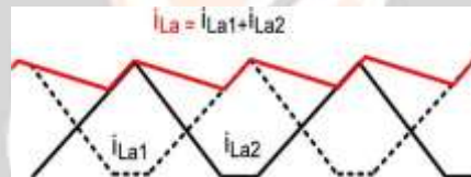
Fig-5: Interleaving between two input inductor currents.
