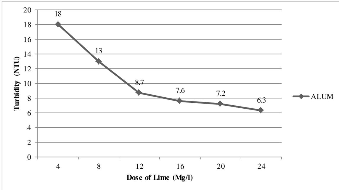
**Figure 5:** Performance of Lime on removal of turbidity at different dose
