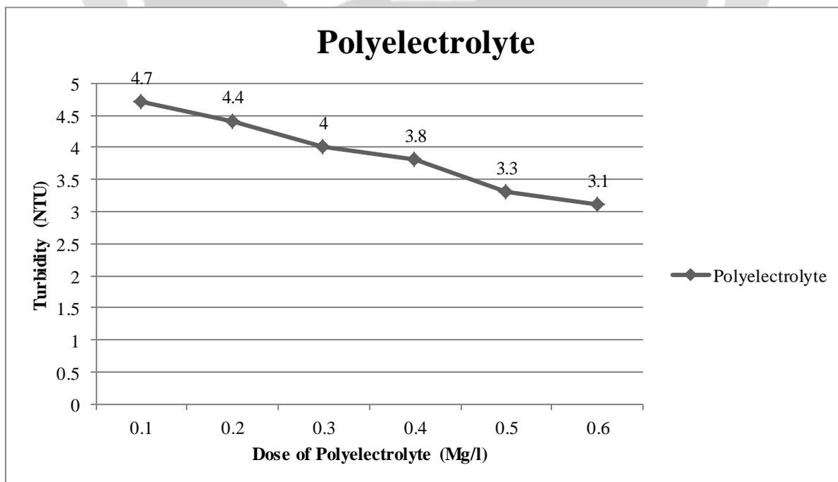
**Figure 4:** Performance of Polyelectrolyte on removal of turbidity at different dose
