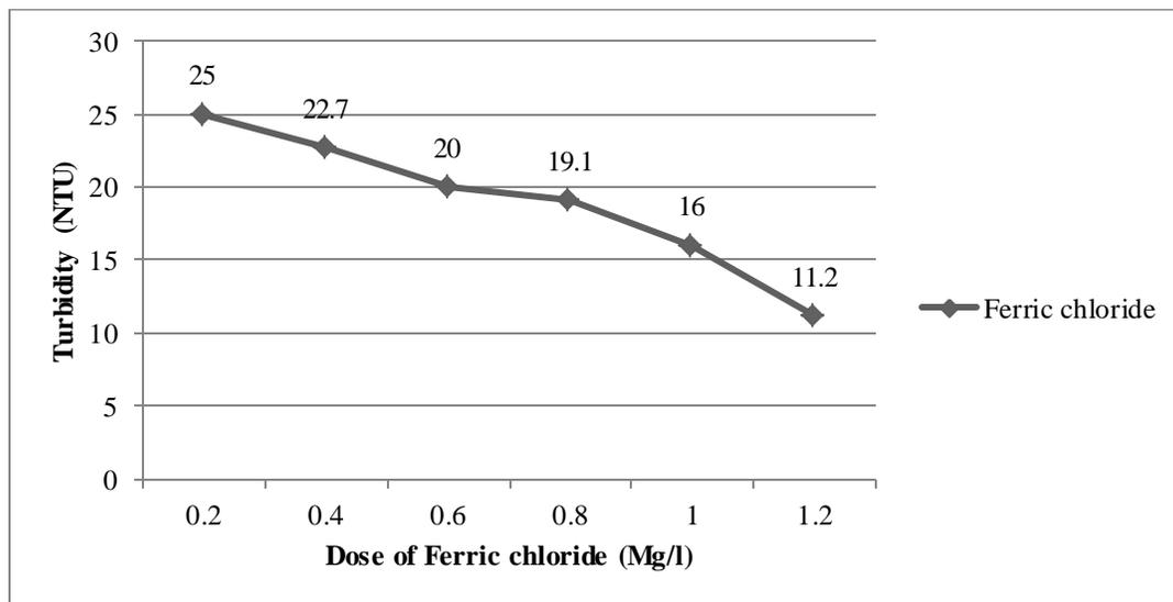
**Figure 3:** Performance of FeCl<sub>3</sub> on removal of turbidity at different dose
