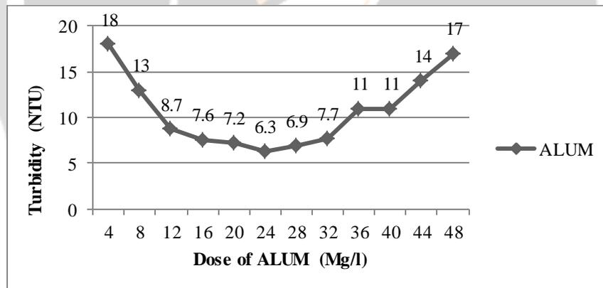
**Figure 2:** Performance of Alum on removal of turbidity at different dose
