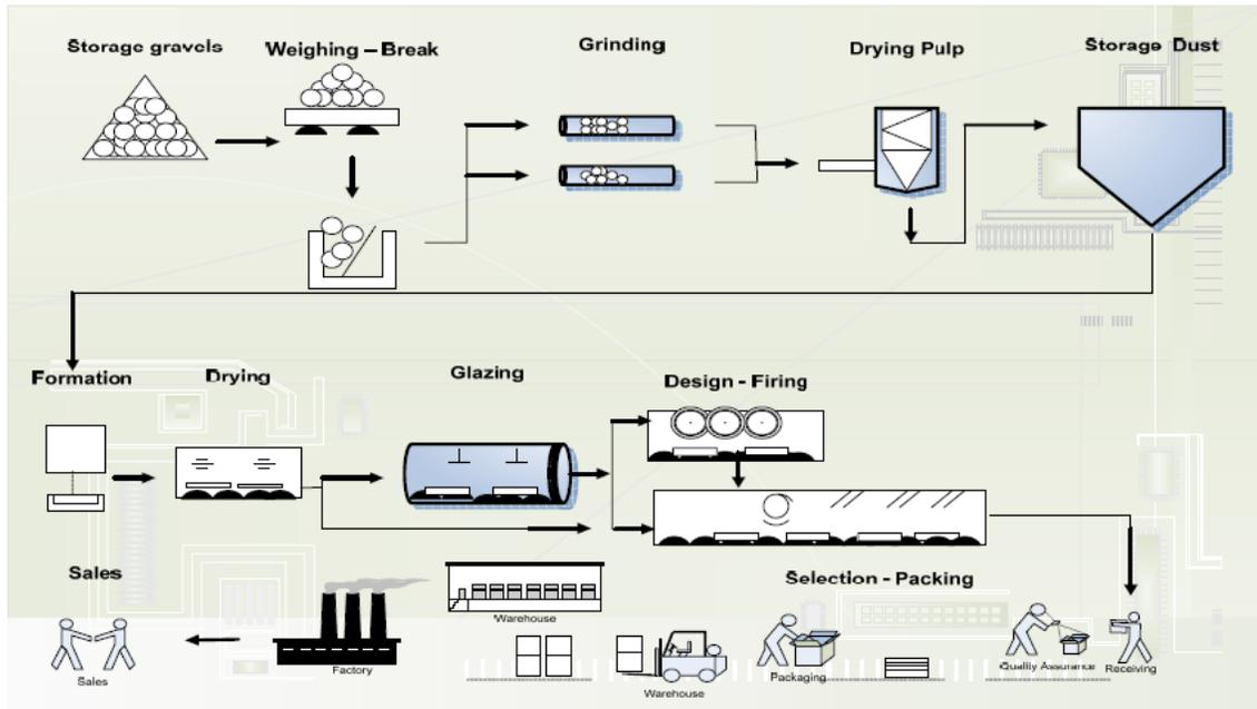
Figure 1: Production process of Ceramics Tiles [1]
