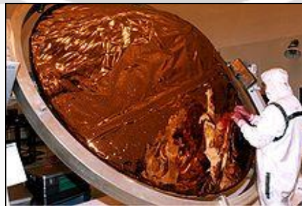
Fig. 4: Thermal insulation on the Huygens probe
