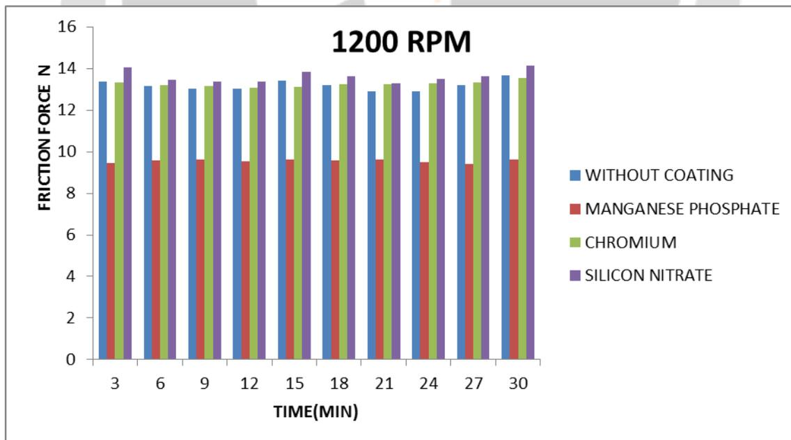
Fig- 11 friction force for different material at 1200 rpm
