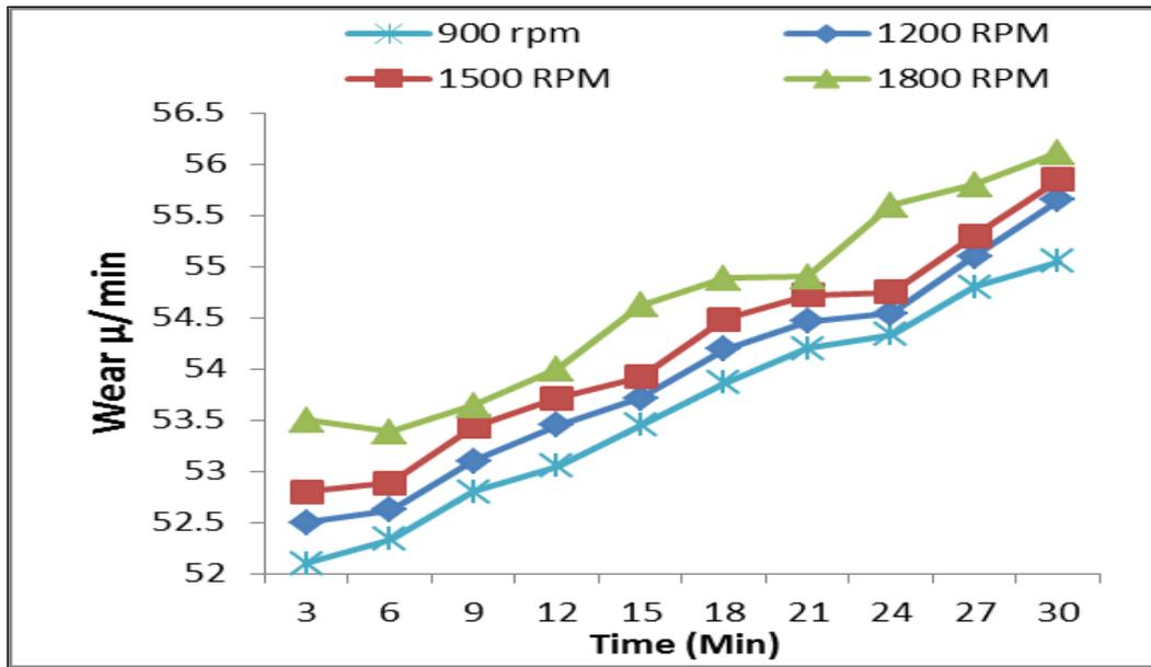
Fig- 8 wear rate for with manganese silicon nitrite coating
