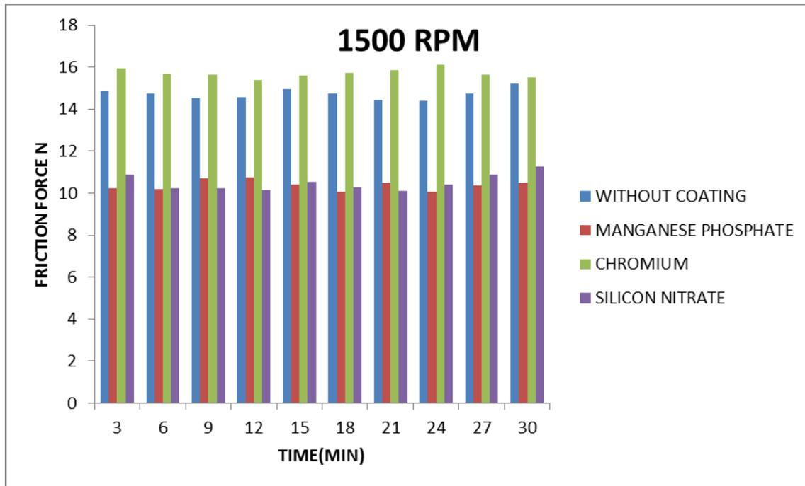
Fig- 12 friction force for different material at 1500 rpm
