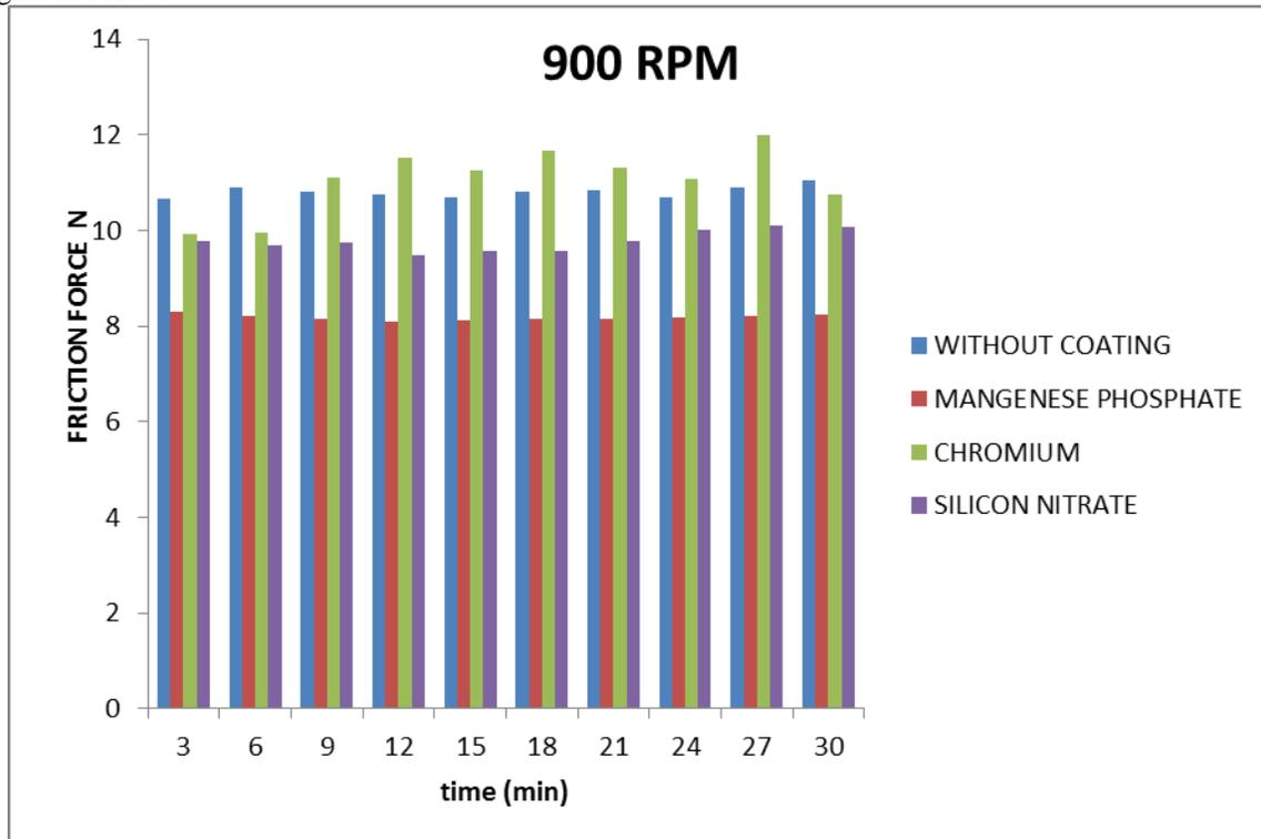
Fig- 10 friction force for different material at 900 rpm
