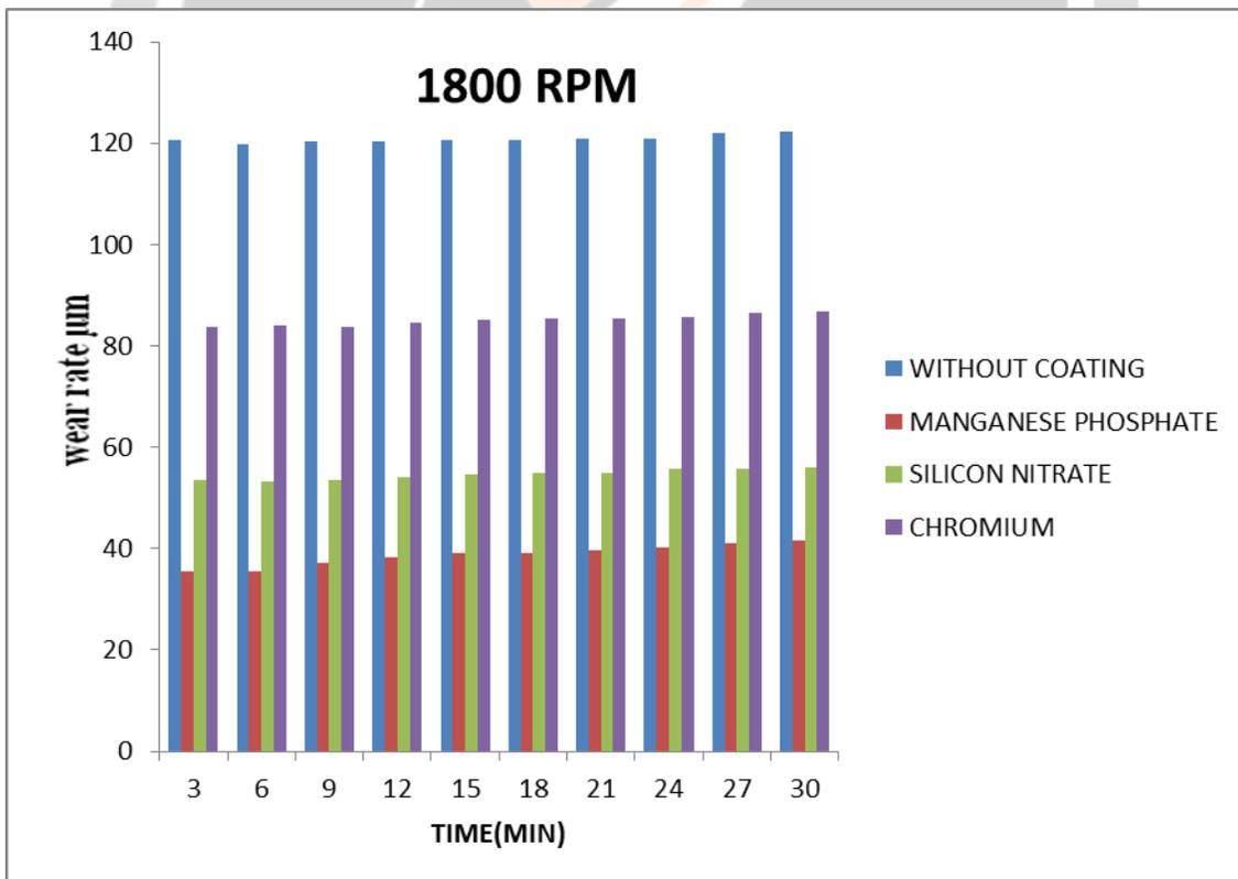
Fig- 17 wear rate for different material at 1800 rpm
