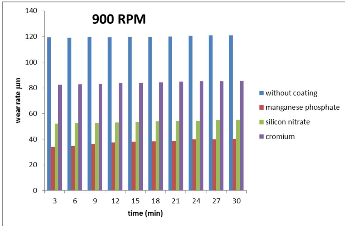
Fig- 14 wear rate for different material at 900 rpm
