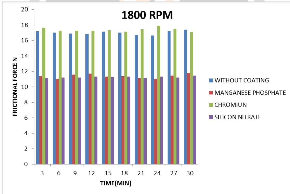
Fig- 13 friction force for different material at 1800 rpm
