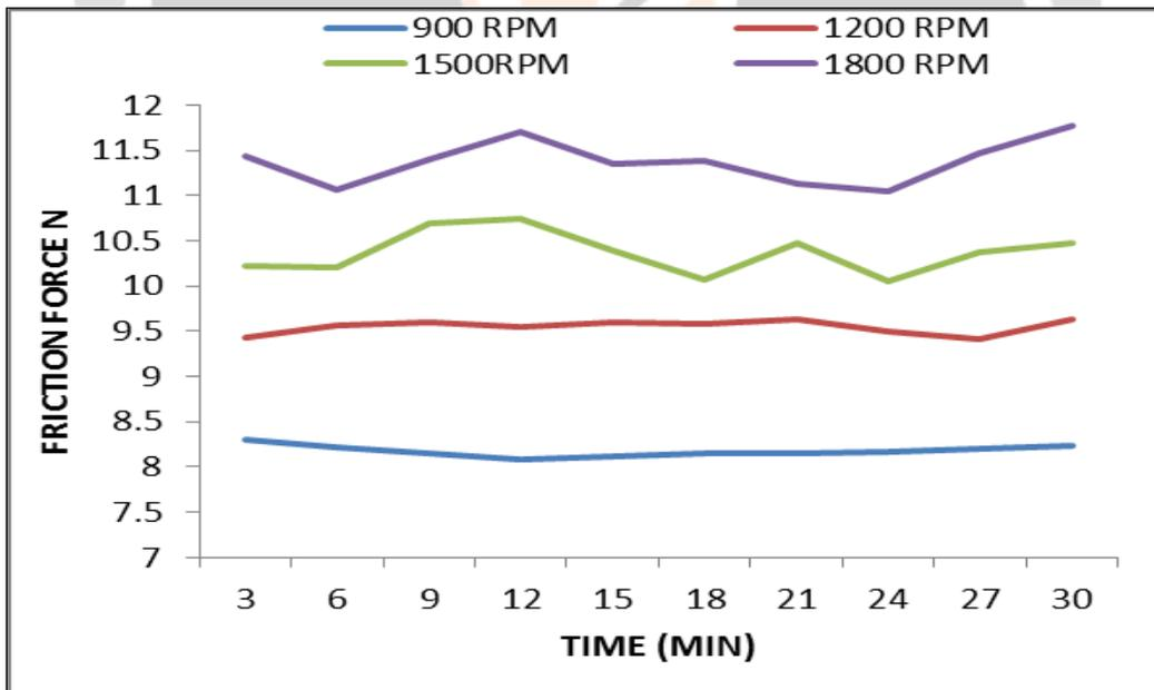
Fig- 7 Friction force for with manganese phosphate coating
