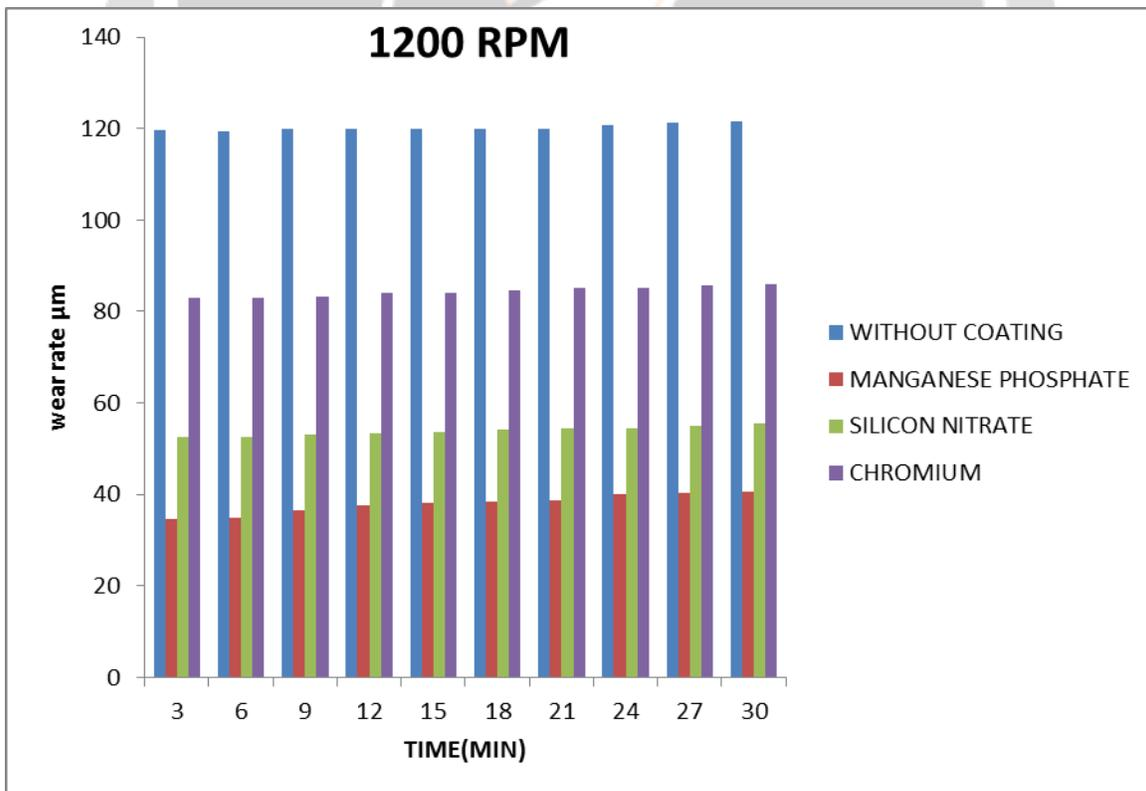
Fig- 15 wear rate for different material at 1200 rpm
