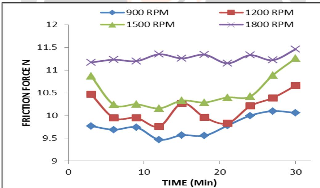
Fig- 9 Friction force for with manganese silicon nitrite coating
