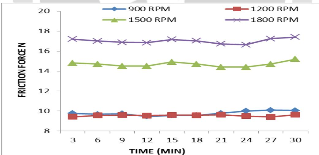
Fig- 3 Friction force for without coating
