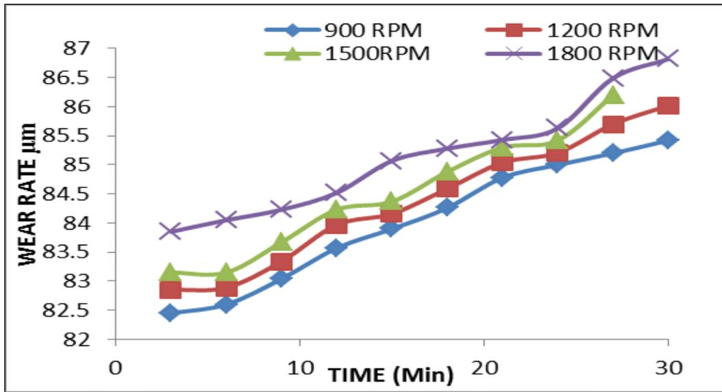
Fig- 4 wear rate for with Chromium coating
