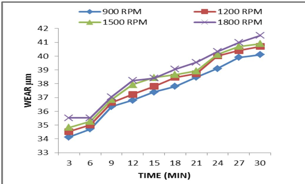
Fig- 6 wear rate for with manganese phosphate coating
