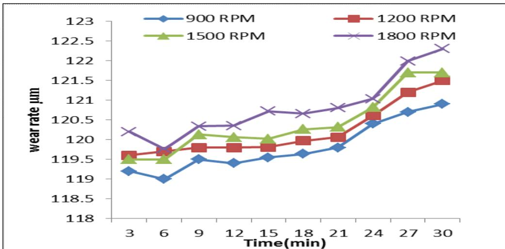
Fig- 2 wear rate for without coating
