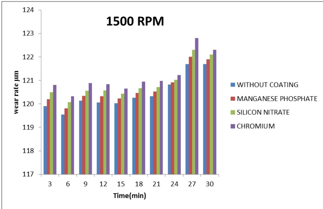
Fig- 16 wear rate for different material at 1500 rpm
