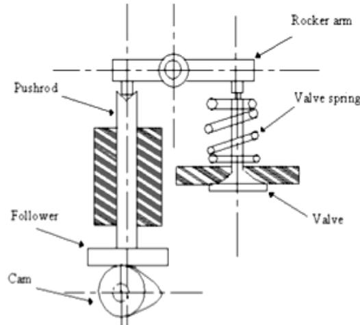
**Fig- 1 Schematic diagram of pushrod type valve train system with flat-faced follower**
