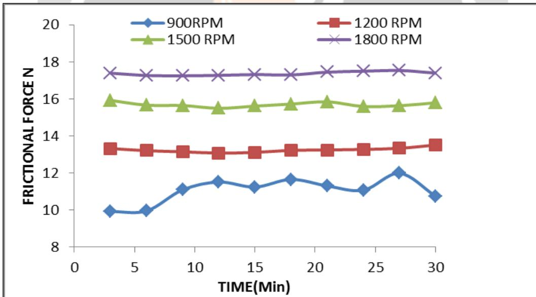
Fig- 5 Friction force for with Chromium coating
