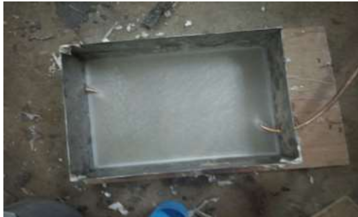
PCM HEAT EXCHANGER
