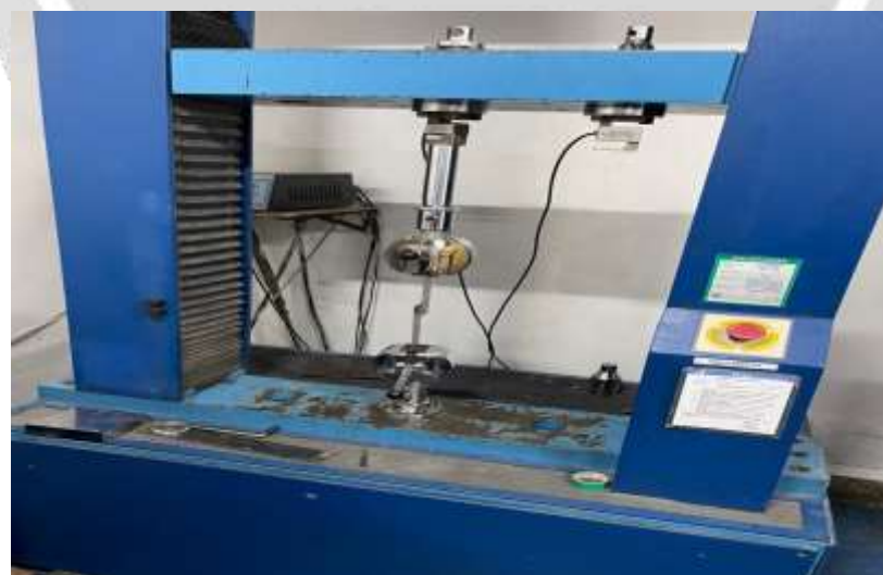
Fig. Testing for rivet joint
