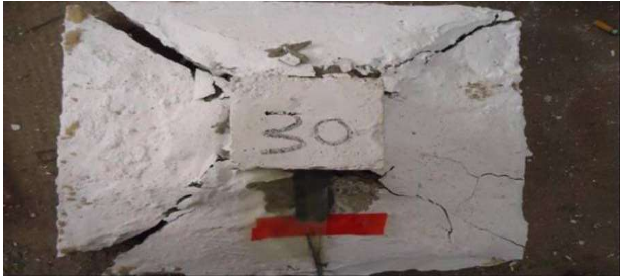
Fig. 4.4 Failure of 30 degree folded footing during a constant load
