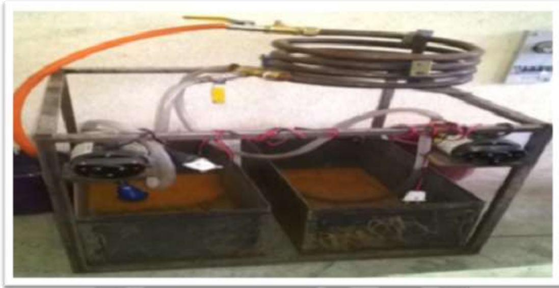
Fig.3 Experimental-Setup Tube-in-Tube Helical Coil Heat Exchanger
