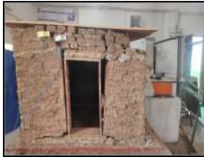
Fig 5: - Model A1 on Shake Table
