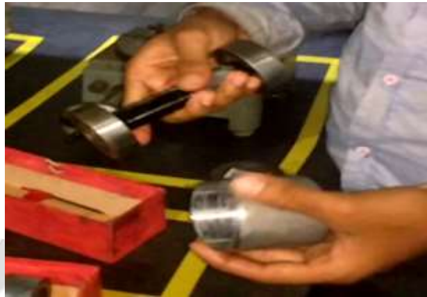
Fig- 7: Go And No Go Gauge
