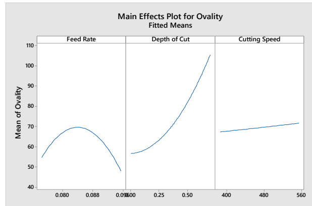
Fig- 13: Main Effects Plot for Ovality Vs Feed Rate, Depth of cut, Cutting Speed
