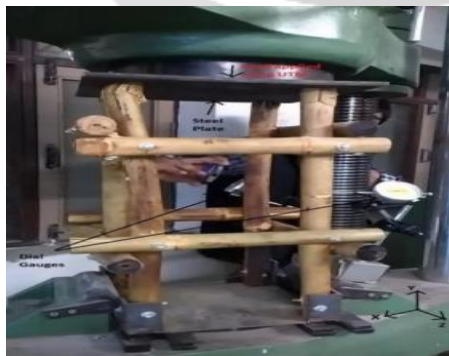
Fig -3: Arrangement of Frame
