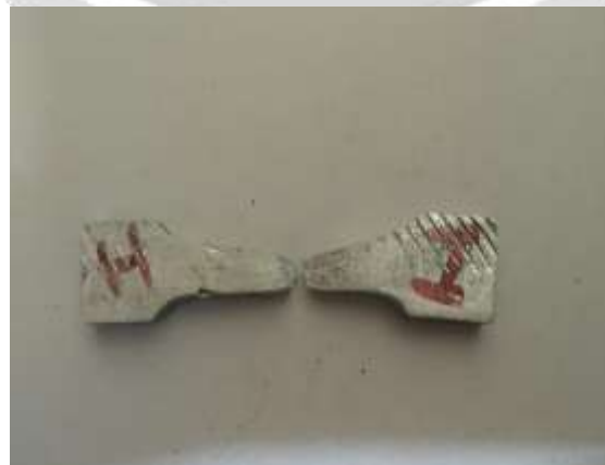
Fig-2 Tensile test specimen after the test
