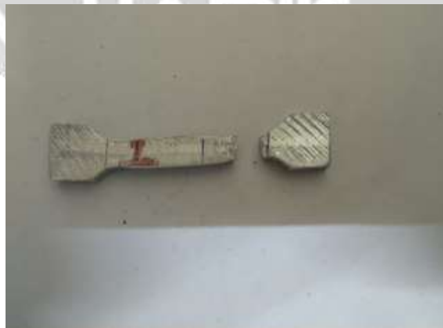
Fig-3 Tensile test specimen after the test
