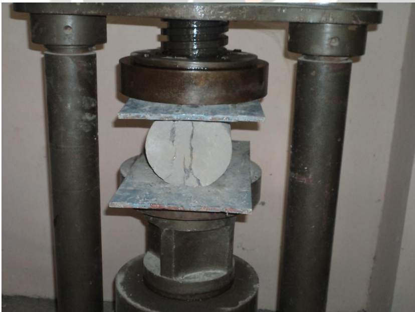
Fig. 7: Split tensile test on concrete
