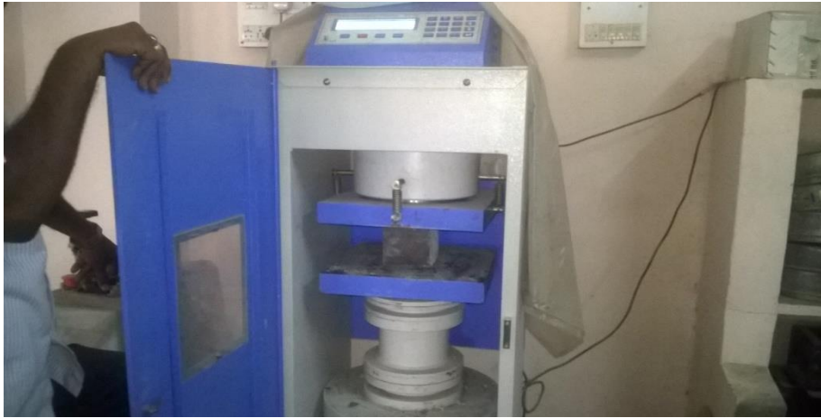
Fig. 6: Compression test on concrete
