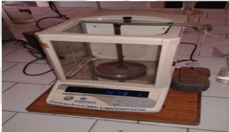
Fig 6: Experimental set up for density measurement
