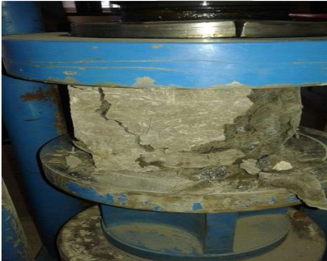
Fig: 4 Testing of Concrete by Compressive Testing Machine
