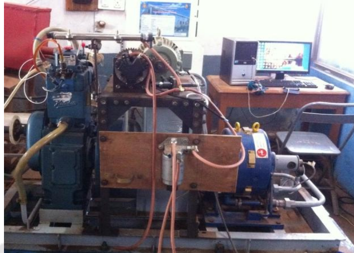
Fig-2: Computerized diesel engine setup
