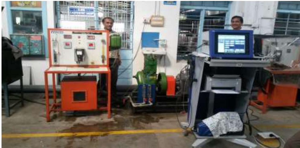
Figure: 2.6 Diesel Engine Test Rig with AVL DiTEST (Exhaust gas analyzer)
