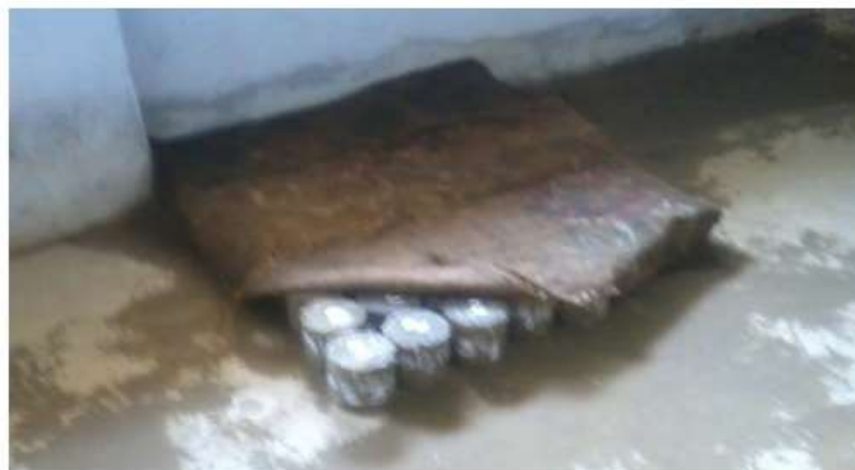
Figure 4.10: Curing of specimens in progress
