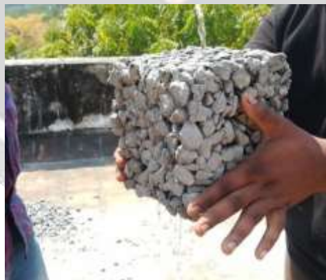
Fig 8: Water Passes Through Pervious Concrete Cube.
