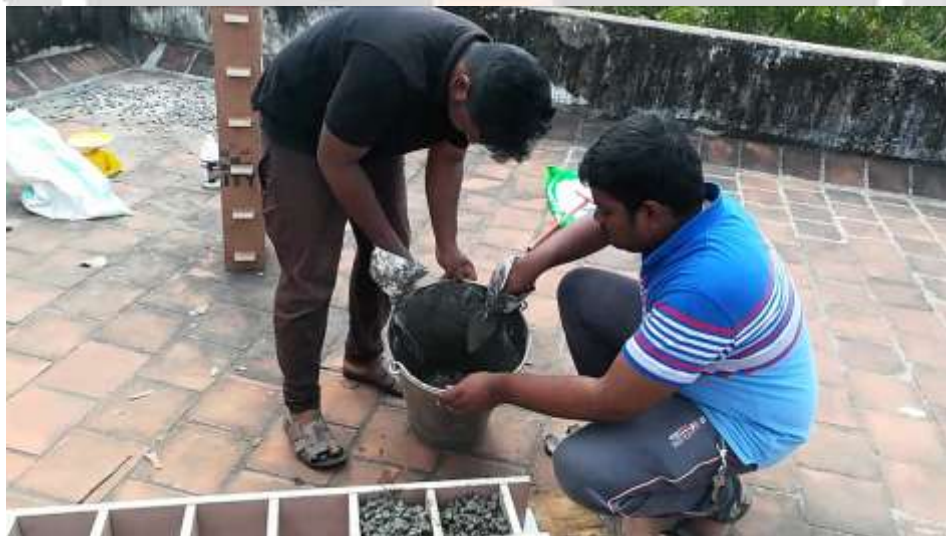
Fig 2: Preparation of Pervious Concrete Cubes
