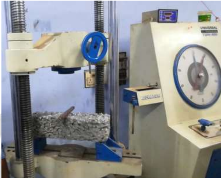
Fig 5: Flexural Strength Test on Prism
