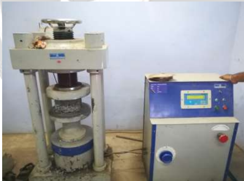
Fig 4: Compressive Test on Cube
