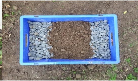
Figure 4: Vertical flow reed bed
