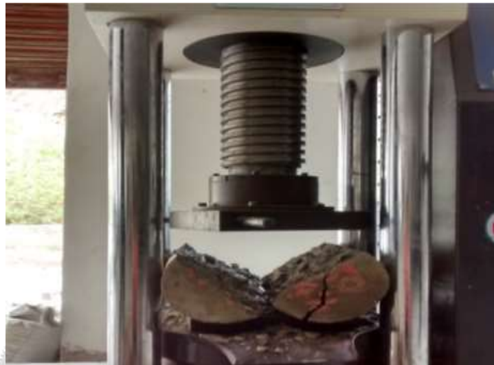
Fig No.2.4. Testing of Cylinder
