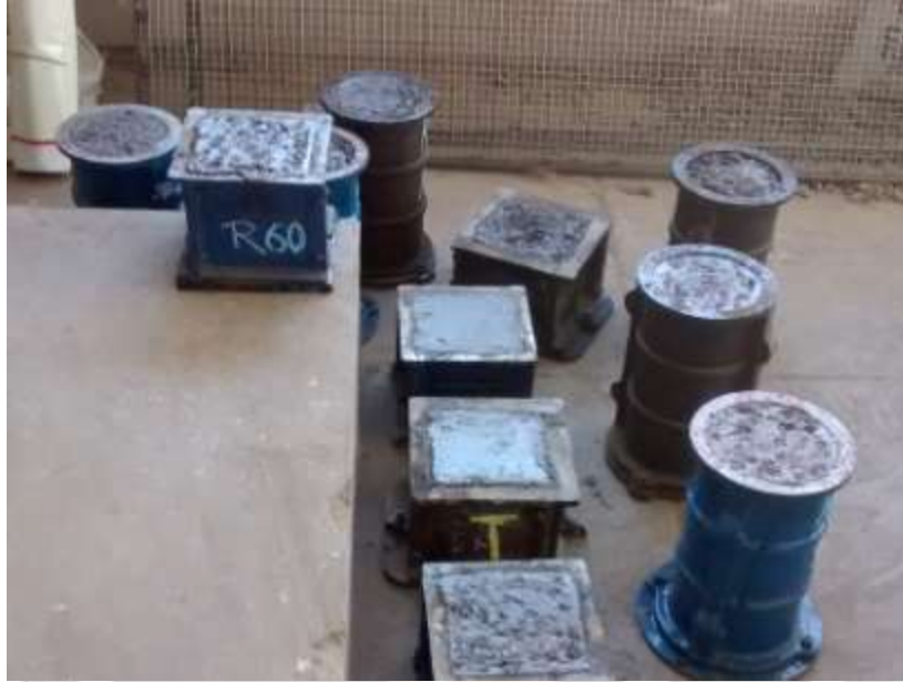
Fig No.2.2.Casting of specimens
