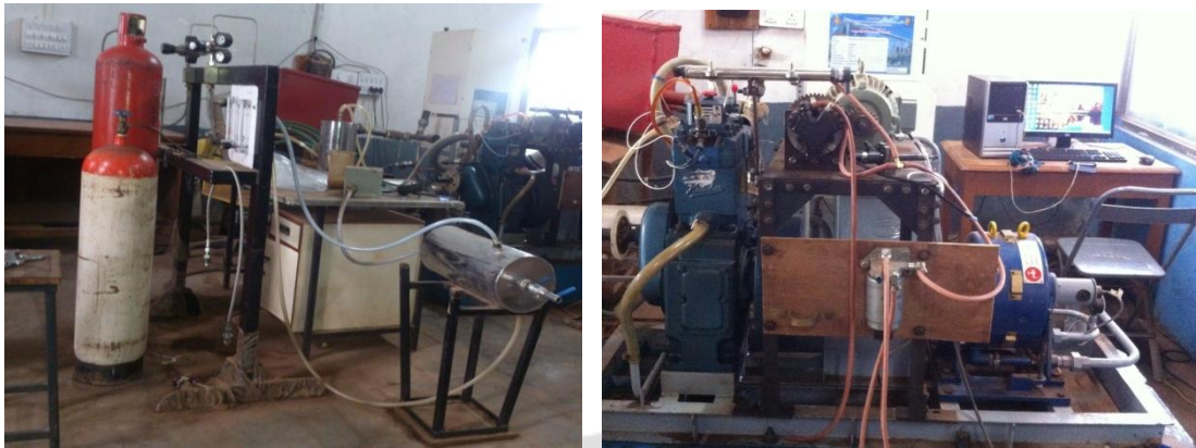
Fig 2 & 3: Computerized diesel engine setup.
