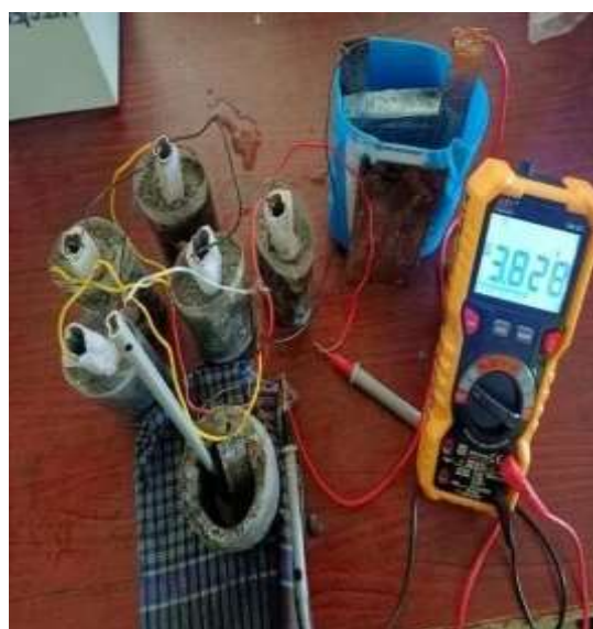
Figure 8: Voltage at starting in the Absence of air
