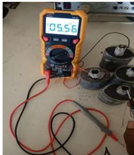
Figure 11: Increase in current in the presence of air
