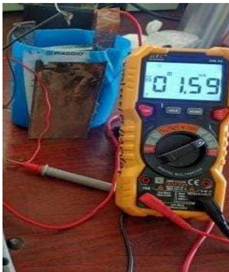
Figure 6: Current at starting in the Absence of air
