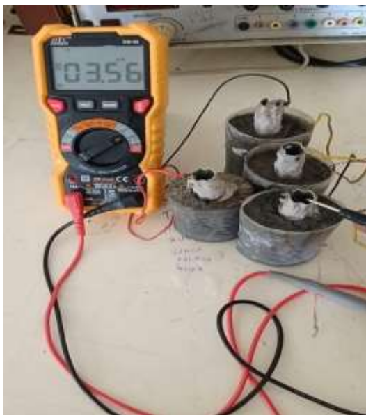
Figure 10: Current at starting in the Absence of air
