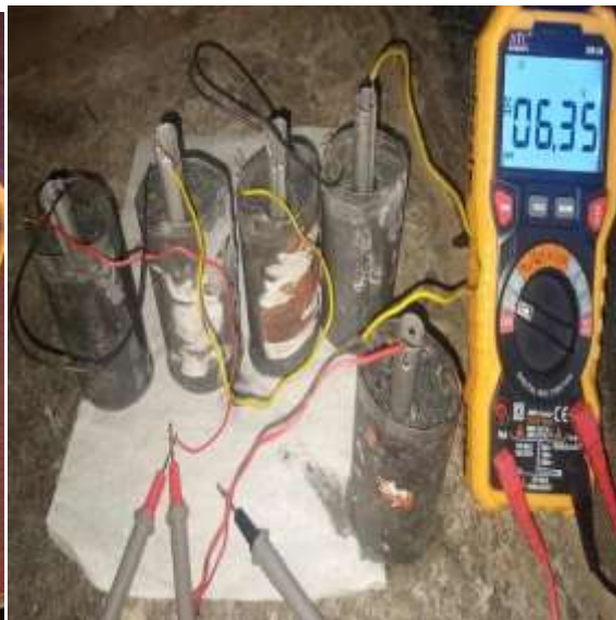
Figure 9: Increase in voltage in the presence of air
