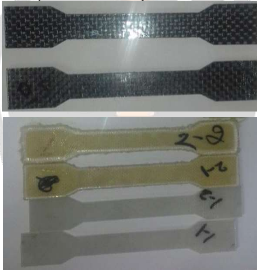
Fig -8: Tensile test specimen of different fibers
