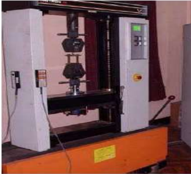
Fig -14: Experimental set up of flexural strength test
