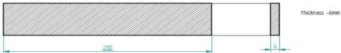
Fig -12: Bending test specimen dimension
