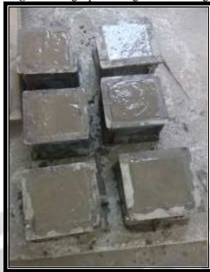
Fig.4 Photograph during cube casting
