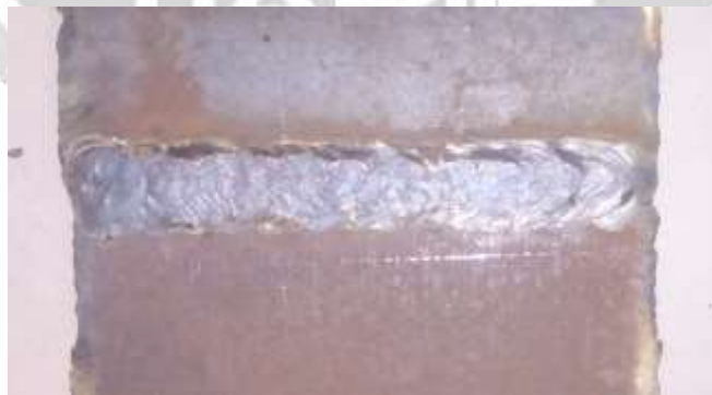
Fig.2 Macrograph of the welded sample (Experiment No.26)
