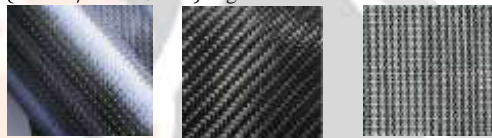
Fig. 14 .CFRP (one-way, two-way, four-way) respectively
