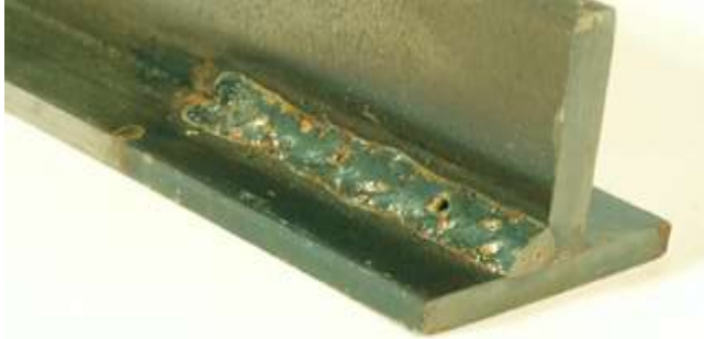
Fig.4 No Shielding Gas – A lack of or inadequate shielding gas is easily identified by the porosity and (pinholes) in the face and interior of the weld.
