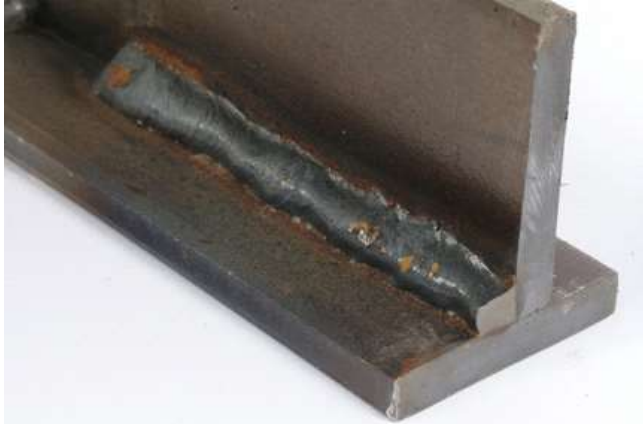
Fig.6 Voltage Too Low – Toolittle voltage results in poor arc starts, control and penetration. It also causes excessive spatter, a convex bead profile, and poor tie-in at the toes of the weld.
