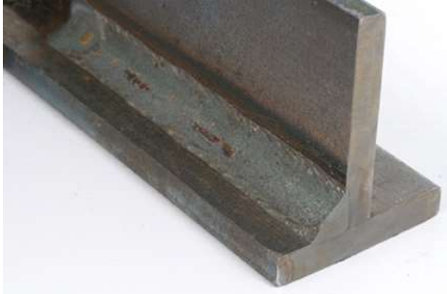
Fig.7 Wire Feed Speed/Amperage Too High – Setting the wire feed speed or amperage too high (depending on what type of machine you're using) can cause poor arc starts and lead to an excessively wide weld bead, burn-through and distortion.
