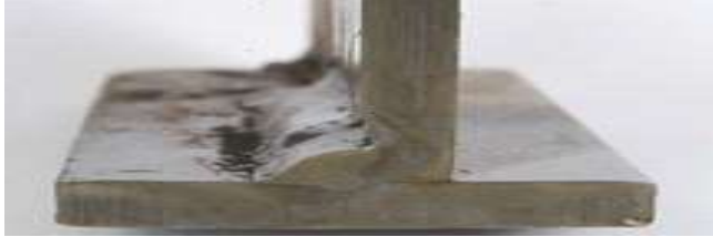
Fig.5 Voltage Too High: Too much voltage is marked by poor arc control, inconsistent penetration, and a turbulent weld pool that fails to consistently penetrate the base material.
