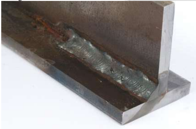
Fig.7 Wire Feed Speed/Amperage Too High – Setting the wire feed speed or amperage too high (depending on what type of machine you're using) can cause poor arc starts and lead to an excessively wide weld bead, burn-through and distortion.
