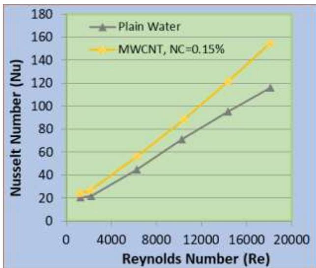
Figure 4: Nusselt Number Versus Reynolds Number at Volumetric Concentration of 0.15%
