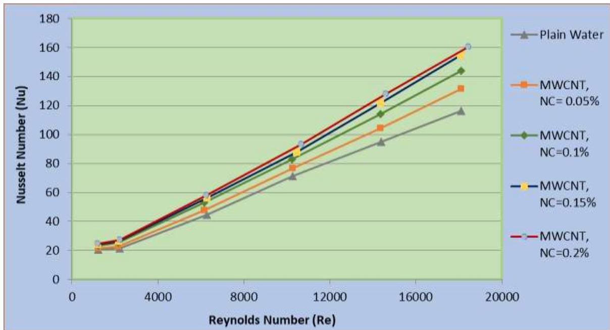
**Figure 6: Nusselt number versus Reynolds number for water and MWCNT nanofluid at varied volumetric concentrations**
