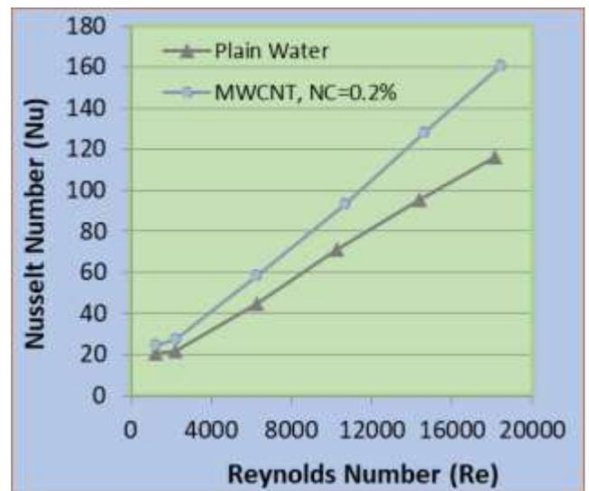
Figure 5: Nusselt Number Versus Reynolds Number at Volumetric Concentration of 0.2%
