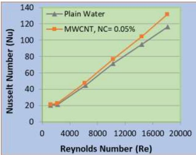
Figure 3: Nusselt Number Versus Reynolds Number at Volumetric Concentration of 0.05%
