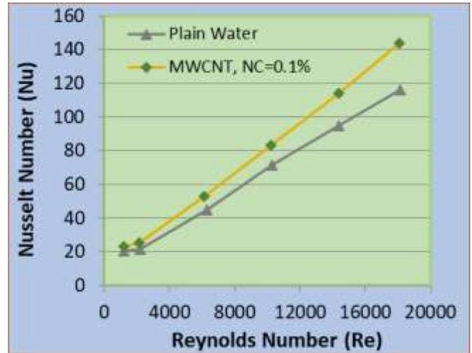
Figure 2: Nusselt Number Versus Reynolds Number at Volumetric Concentration of 0.1%
