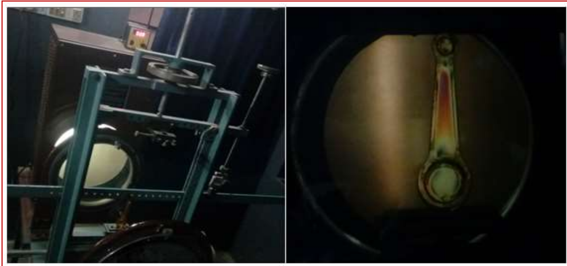
Figure: 4.2 Experimental setup, Compressive and tensile load acting on the both ends of connecting rod specimen.
