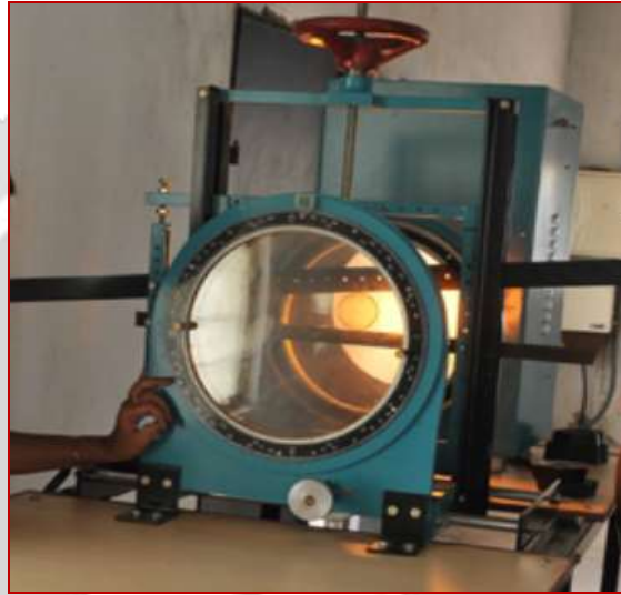
Figure.4.1 Calibration of Photoelastic sheet on circular disc.
